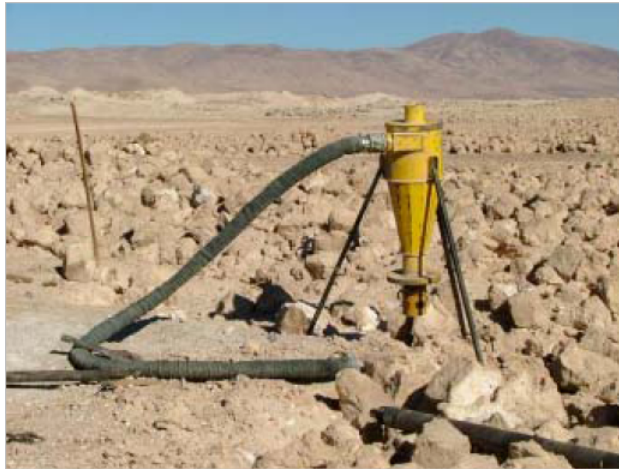
cyclone collecting sample during drilling
